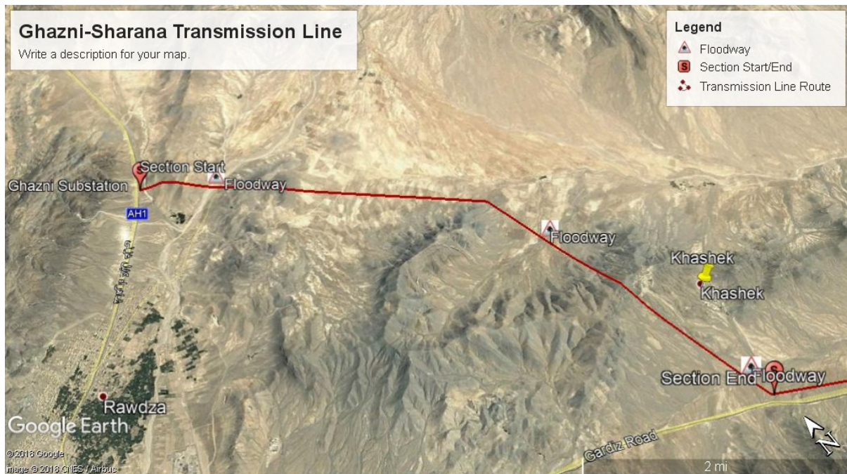
Figure 4 Ghazni Substation to Gardez Road near Khashek village (0-10 KM) section of the transmission line.
